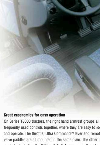
frequently used controls together, where they are easy to identify and operate. The throttle, Ultra Command™ lever and remote valve paddles are all mounted in the same plain. The other major controls, including the PTO switch, linkage and draft controls, transmission control modes and traction management, are all grouped within a separate lower section of the same armrest. This logical layout is easy to learn and simple to use.
