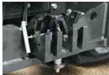
The heavy-duty Reynolds Quick Hitch drawbar is engineered exclusively for T9000 scraper models. In concert with the T9000 "center-pull" design, the drawbar provides a superior pull angle for efficient pulling power. It comes standard with an attached tow cable on scraper models.
