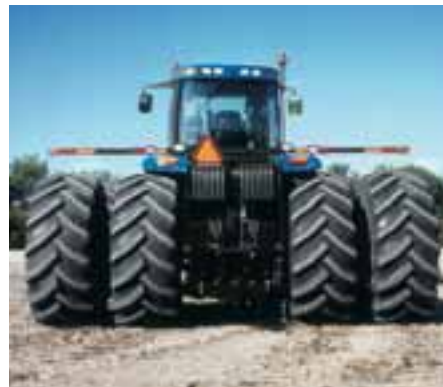
Larger tire options increase traction efficiency while reducing compaction, for improved yields and productivity. Since frame size is matched to horsepower for optimum performance, additional weight doesn't have to be added to T9000 tractors for many applications. In applications requiring extra ballast, a front cast weight bracket can be added to the frame for additional ballast with up to 18 suitcase weights. Suitcase weights and a cast bracket can be added to the rear of T9000s without a three-point hitch. Wheel weights are also available for the front and rear axles.
