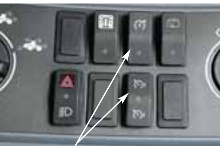
Use the Constant Engine-Speed switches to set the max rpms and the speed adjustment switch or throttle to return engine speed to the desired level after making a turn.
