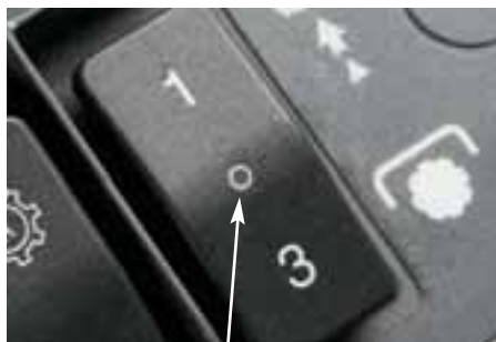
For scraping in large-scale commercial applications, the Precision Land Management Integrated Laser Leveling System allows the tractor's electronics to automatically control depth on the first and third remotes.
