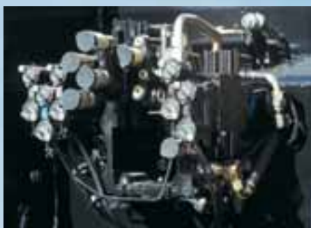
Up to nine remote valves and MegaFlow™ can be built into any T9000 model. Seven remote valves and power beyond are pictured.
