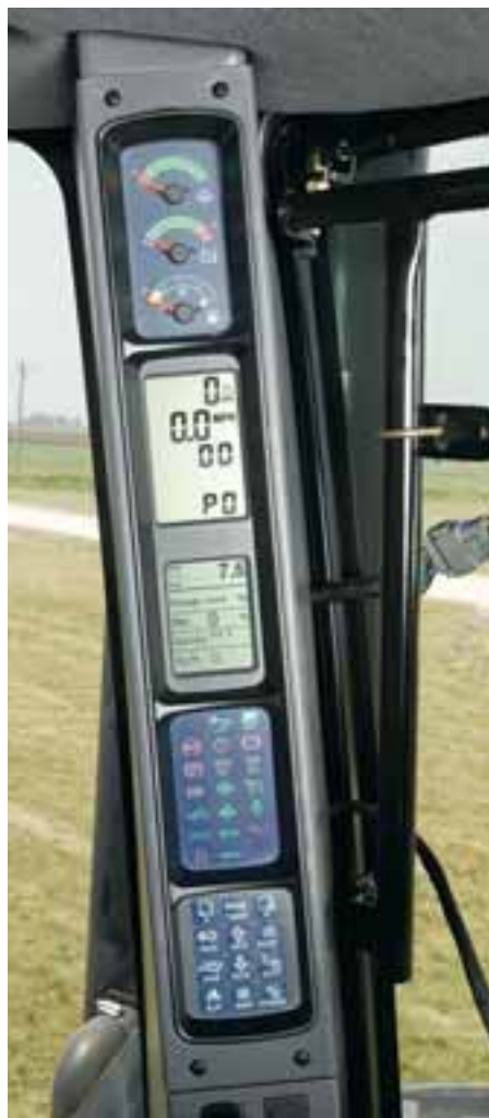
All the information you need “on the go” and at a glance—you can monitor everything from wheel slip and ground speed to fuel usage and hydraulic-flow readings with performance instrumentation that’s integrated into the cab post for easy viewing (standard on Ag and HD Ag models equipped with powershift).
