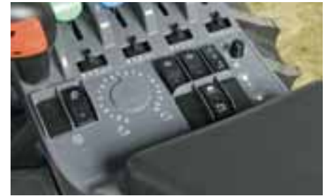
Differential locks have independent controls for front and rear axles.
