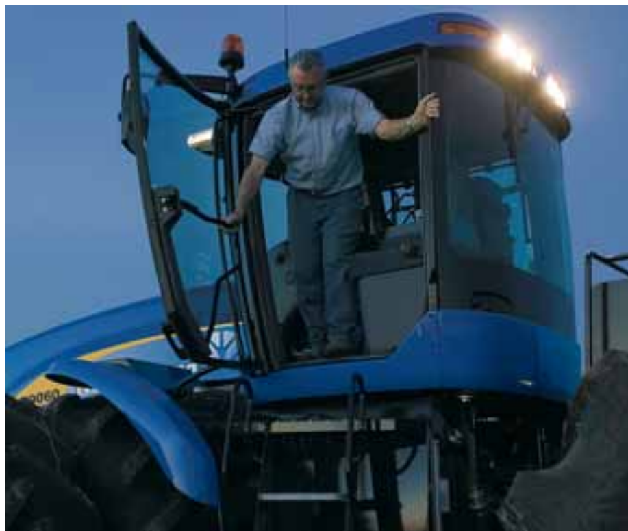
Convenient egress lighting lets you safely exit the cab when it’s dark.
