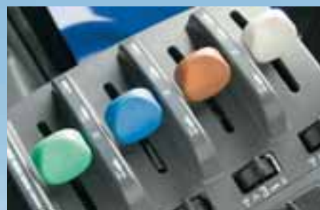
Hydraulic control levers and couplers are conveniently color-coded for ease of hook-up and to help track hydraulic operations.
