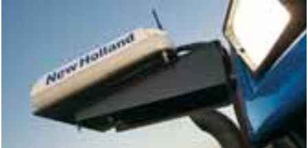
The New Holland antenna receives the GPS signals to guide the vehicle. This antenna can easily be transferred from tractor to tractor or even to your combine.
