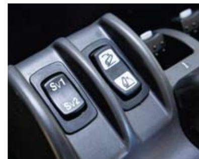
As an added benefit, the system has the unique ability to couple A and B engine speed settings with the ground speed memory system. When activated, this feature allows the operator to alter both the engine speed and the transmission ground speed with the "SV1" and "SV2" buttons.
