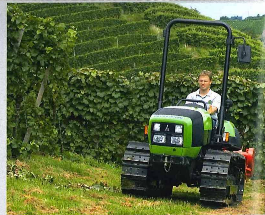
The Agroclimber's slim chassis is particularly well suited for use in vineyards.
