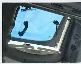
The cab roof incorporates a large glass hatch so that front loading can be performed in complete safety with full visibility.
