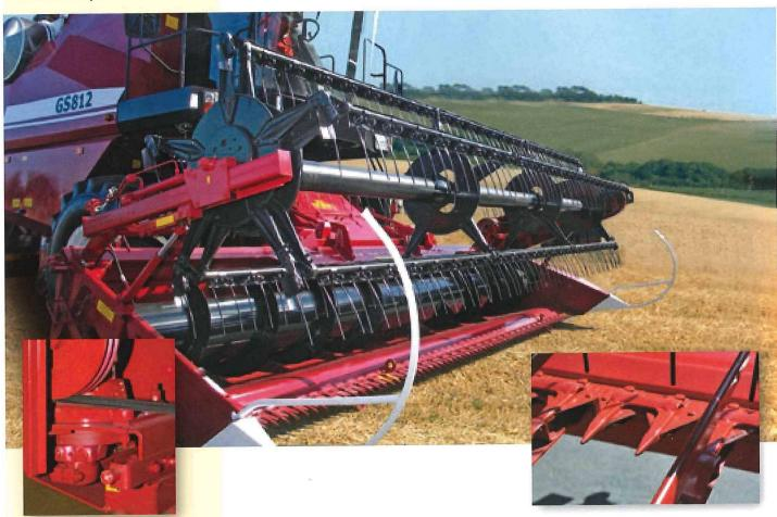
The Schumacher planetary gearbox, which is used to drive the header assembly, ensures a high cutting frequency (1108 strokes per minute) a smooth operation and minimal wear, thus increasing productivity.
