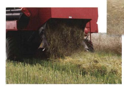
The straw chopper with its increased number of blades thoroughly breaks down the straw and spreads it evenly over the field in the specified width as a fertilizer, creating a good basis for future crops.
