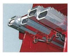
Optimal distances between the height of the stages and the intense movement of the shaker ensures almost complete separation of the remaining grain from the chaff.
