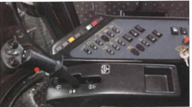
The speed control handle fits easily and comfortably into the operator's hand and it includes adjustable palm rest. The handle is placed on the auxiliary counter and it simultaneously controls the seat so that it stays within easy reach. It permits single handed control functions necessary for quick decision-making - forward and reverse, speed, position and speed of the header drum, position of the conveyor of feeding channel and momentary disconnection of its drive.
