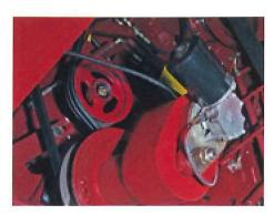
Electrical purging fan speed control from the cabin: optimal settings for various plant crops and harvest conditions.
