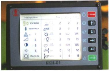
Once switched on, the on-board computer will automatically check the sensors and mechanisms to ensure reliability and it has circuit diagrams with circuit numbers and advice on troubleshooting.
