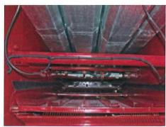
The three stage grain purifying system, with a sieve area of almost 4 m2 is an optimal solution for a mid-class harvester.
