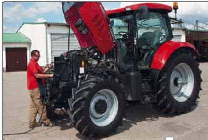
Easy daily checks and cleaning: with new swing out coolers. Similarly the air filter is conveniently situated for quick inspection. Should you only be checking the oil level, this can be done with the hood closed.
